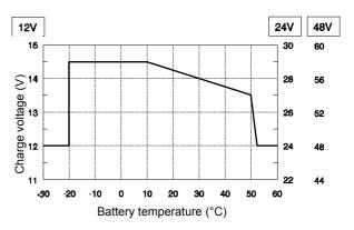
Figure 4: Temperature compensated charging
