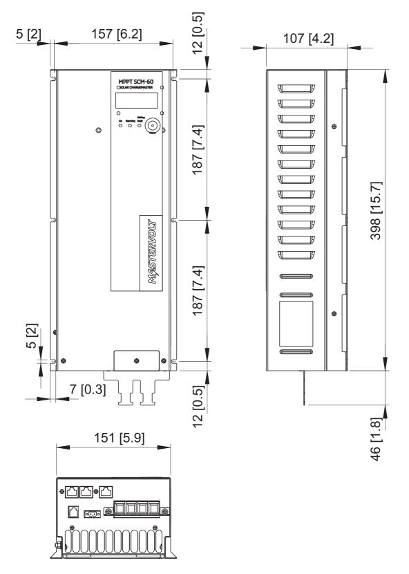
Figure 22: Dimensions of the Solar ChargeMaster in mm [inches]
