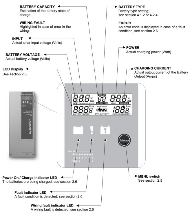
Figure 5: operation of the Solar ChargeMaster
