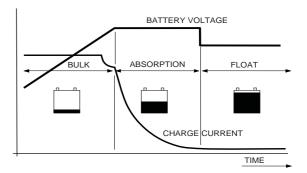
Figure 3: Three step charge system
